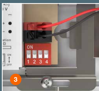
DIP switch for easy power steps setting.
